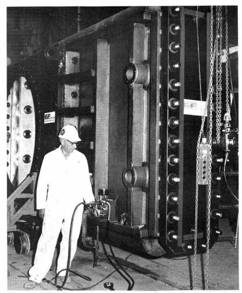
TO CLOSE AN OPENING across a six-foot-diameter line-of-sight pipe, Dept. 1130 came up with two overlapping 12-inch-thick gates which achieve closure in 35 milliseconds. Here Dick Teisher (1130) examines one of the gates, tested in the MINERS IRON experiment in Oct. 1980.
